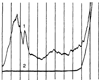
Figure 5 Reduction of manganese dioxide of the rutile type. Twelve millilitres of 0.2 M \text{H}_2\text{SO}_4 + 6 mg \text{MnO}_2 (1), Electrically stirred suspension (2), Quiet suspension. Sensitivity 1/1000, beginning from 0 V, 200 mV/absc (Reproduced with permission from reference 18)
